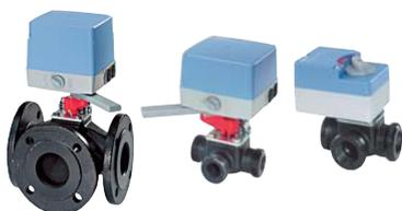
Motorized slipper valves for basic applications in smaller heating systems. 3- and 4-port slipper valves are ideally suited for small, easy-to-control heating systems with small differential pressures. Both slipper valves and butterfly valves are available with directly coupled rotary actuators. These motorized valves can be installed in no time since linkages are no longer required, representing affordably priced solutions.
